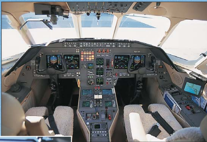
(Top) The 2000 offers a Collins Pro Line 4 panel. (Left) A Flight Dynamics HGS is a popular option at $483,200. (Right) A spacious 8-pax configuration was featured on this aircraft. (Insert ) There was plenty of headroom even for Lacy.
