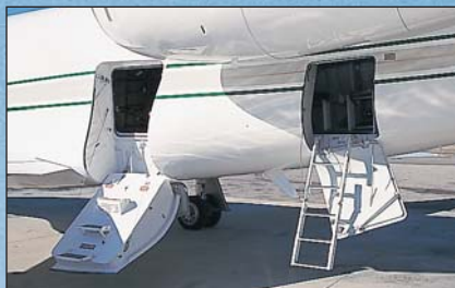
(L) The airstair and entry door of the 2000 are very comfortable. A pair of CFE 738-1-1Bs feature dual FADEC control. (Bottom) Ample baggage storage is available in the 2 aft compartments, each with built-in steps.
