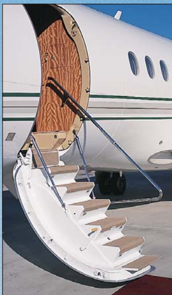
(L) The airstair and entry door of the 2000 are very comfortable. A pair of CFE 738-1-1Bs feature dual FADEC control. (Bottom) Ample baggage storage is available in the 2 aft compartments, each with built-in steps.
