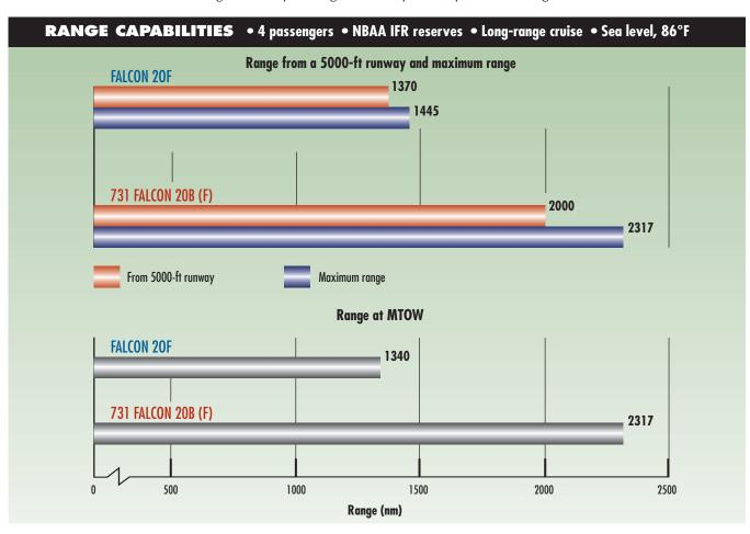
With the retrofitted AlliedSignal TFE731-5BR engines, range is dramatically increased and DOCs are significantly lowered.
