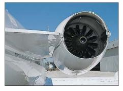
A Collins Pro Line IV five-tube EFIS panel (top) is a popular option on the 731 Falcon 20B upgrade menu. With its 700-cu-ft cabin volume (above), the 20B offers the most spacious airborne accommodations in its class. For \$3.78 million, you can put a pair of 4750-lb thrust TFE731-5BRs (L) on your Falcon 20, which nearly doubles the range capability of the airplane.
