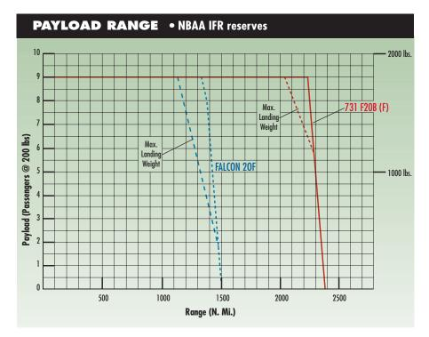
One advantage of the 731 Falcon 20B program is that an operator can load the airplane with full passengers and full fuel and fly 80% farther than a Dassault Falcon 20 could.
