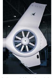
climb. Handzlik explained that with full fuel and two passengers, the EC120B will climb to 10,000 ft in eight min, starting off at about a 1500-fpm climb and stabilizing out
