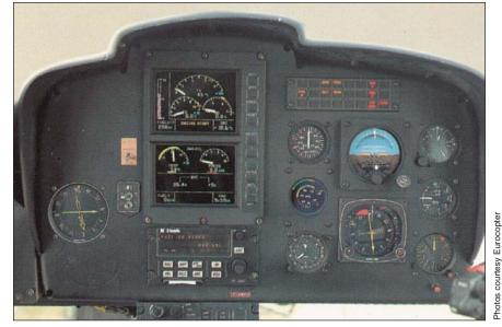
New flightdeck display technology on the EC120B centers around a fully-duplex vehicle and engine multifunctional display (VEMD). First limit indications are clearly presented on takeoff and during normal flight operation to greatly reduce pilot workload.
