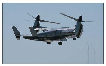
sions. The fuel burn required to hover, however, is more than in forward level flight at 240 kts. So to save fuel, and to operate quieter, you may want to do a running STOL takeoff at 60 to 75 nacelle angle when possible.
