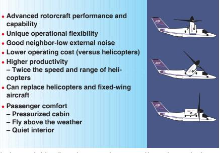
The design goal of the Bell 609 tiltrotor is to acheive King Air-like speed, cruise altitude, passenger comfort and anti-icing attributes coupled with the ability to takeoff and land vertically. quickly, at about 40 kts, and climbed almost vertically as we pulled up at more than 500 fpm.
