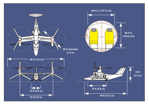
The Bell 609 will be a big airplane, 60-ft wide from tip-to-tip and 14-ft tall, but its mission flexibility will be without equal and cabin comfort will be more than adequate for 8 to 9 pax.
