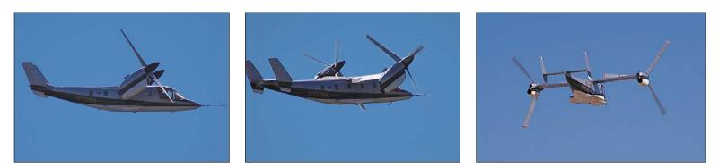
less than one min. Engine tilt control is managed with an easy-to-use "coolie hat" toggle switch on the collective. In "full forward," the XV-15 feels just like an airplane.
