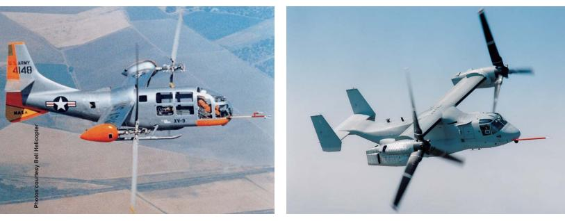
Bell's first tiltrotor, the XV-3 (above L), is shown here during flight testing in the 1950s. Current-day flight trials of the Bell Boeing V-22 Osprey (above R) are well underway with seven aircraft already in the flight test program.
