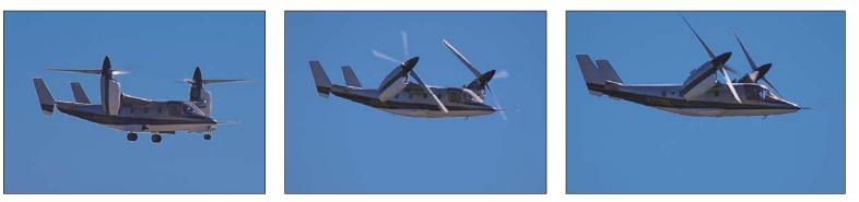
The conversion from a vertical nacelle angle to full-forward airplane mode can be accomplished in as little as 12-sec with a zero to 200-kt acceleration in
