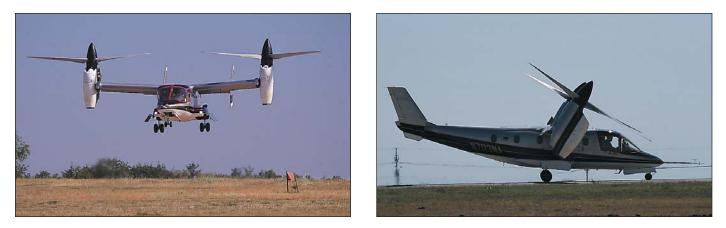
Lacy maneuvers the XV-15 side-to-side using blade tilt (above L). After executing a rolling 20-kt touch-and-go approach to landing (above R), Lacy perfromed a running takeoff with a 60-degree nacelle angle (top photos on opposite page).
