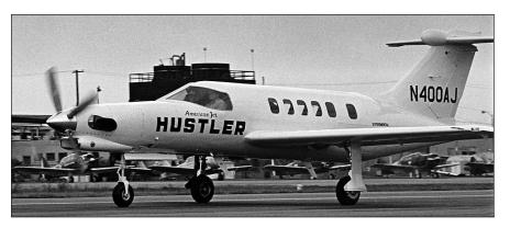
The 1970s Hustler, "a somewhat controversial concept." This airplane was designed for single-pilot operation and was originally planned to have a P&W PT6 turboprop in the nose and a P&W JT15D jet in the tail. The rear-mounted jet was never installed and the Hustler didn't make it into production.
